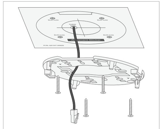
If necessary, install drywall anchors using the alignment sticker. Feed the ethernet cable through the middle opening of the back plate, then fasten the back plate to the mounting surface using the provided screws.
