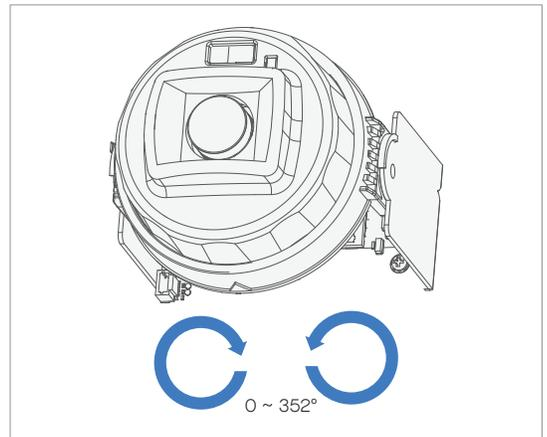
*Optional:* Tilt lens. May need to rotate 180° to tilt in the reverse direction.
