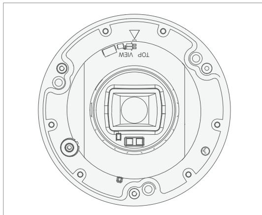
This is the top of the camera and should be mounted with this side up.
