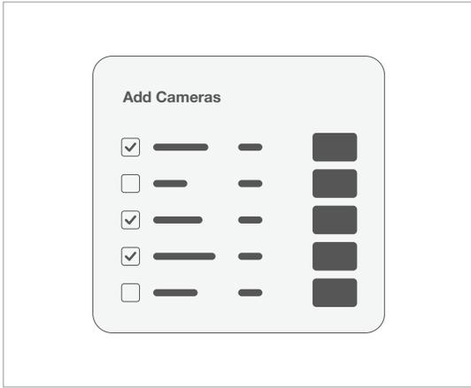
When your camera is plugged into the network, add the camera to your dashboard by going to **Devices > Cameras > Add Cameras**. You can identify your camera in the results via the serial and/or MAC address printed on the camera's box.
