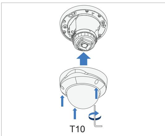
Once the aperture is properly aimed, use the Torx driver to secure the lid.
