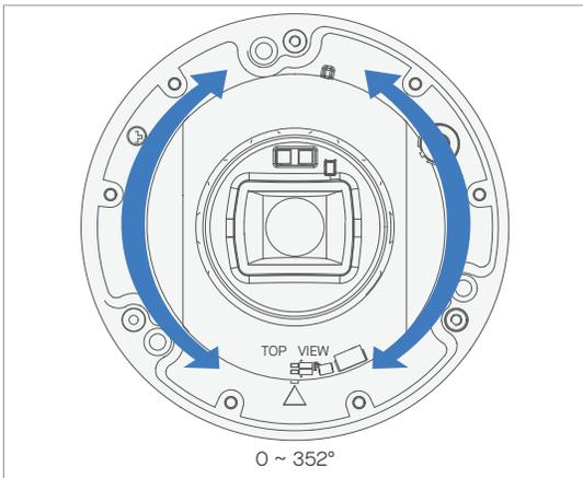
*Optional:* Twist camera base to rotate.
