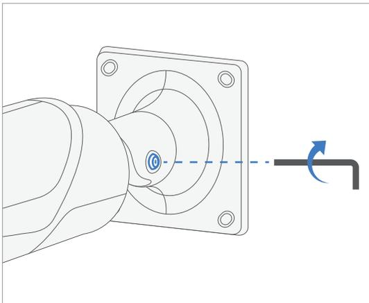
Tighten camera pan screw with Torx driver.
