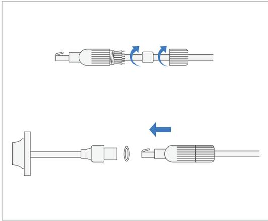
Attach cable gland if using outdoors or in a wet environment.
