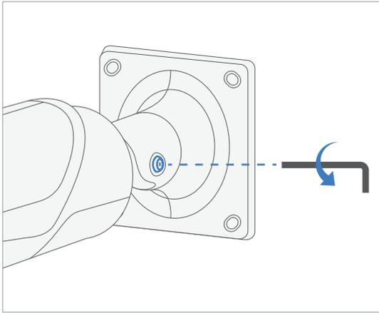
Loosen camera pan screw with Torx driver provided.
