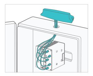
If installing a multiband antenna on the enclosure, drill a %" hole and wipe the surface clean before routing the cables and applying the double sided tape.
