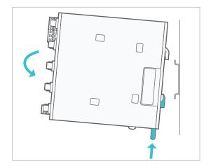
Angle the unit and hook it onto the DIN rail, angle it down and push the latch back up to lock.
