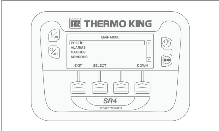
**EN** Please note, once any additional Thermo King telematics hardware has been installed, the reefer HMI will need to be configured for 3rd party access and remote control. Please work with your local Thermo King dealer to update to the correct 3rd party integration configurations in the guarded access menu.
