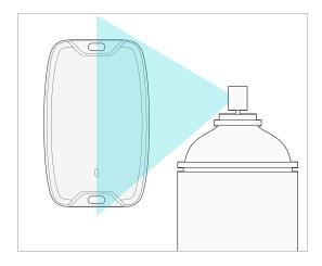
(Optional) Spray paint the device to camouflage it but do not use a metallic paint which might interfere with antenna performance.
