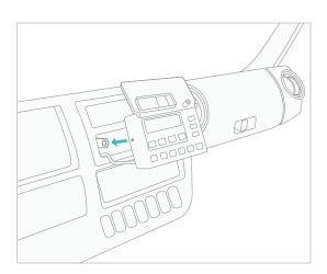
Fasten connected gateway in a secure position. Verify the gateway indicator light turns green, this could take 1-3 minutes.
