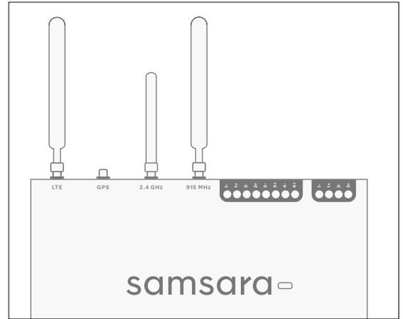
Attach the antennas to their corresponding connectors at the top of the controller.
