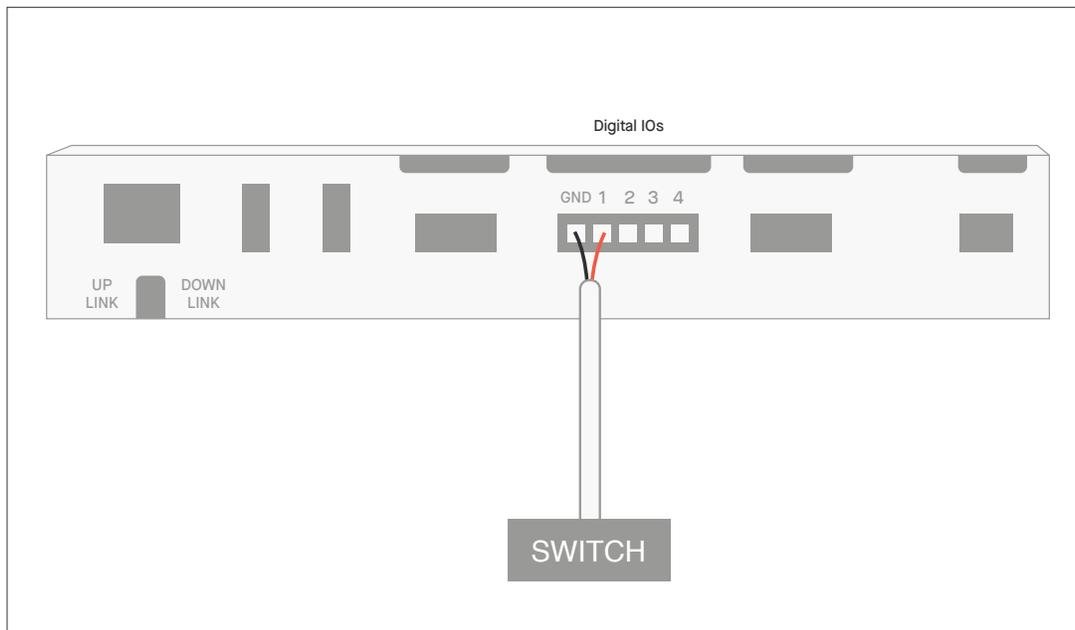
Connect the input to both GND and the desired terminal (1-4).
