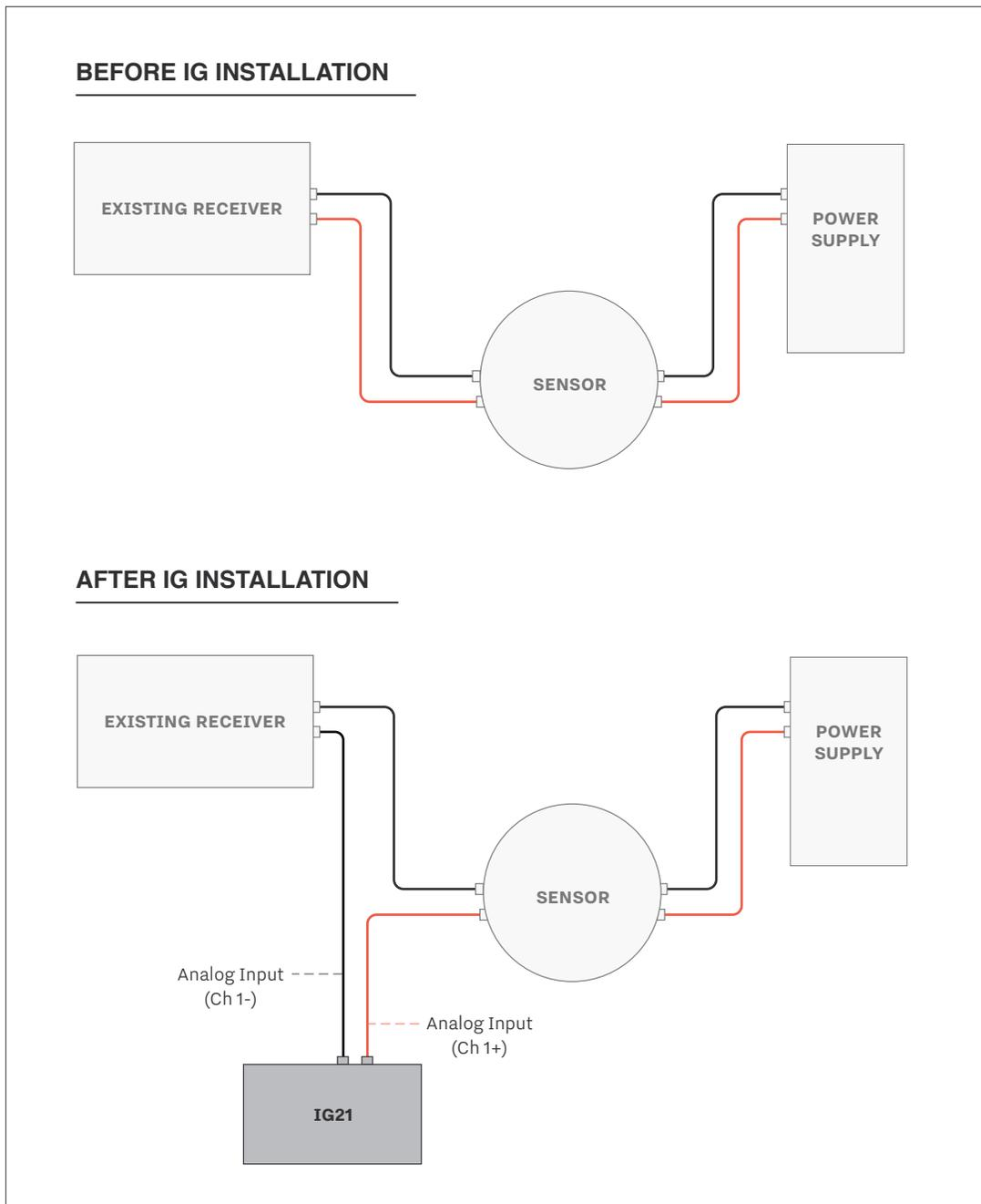
Recommended wiring for adding the IG to an existing current loop with an existing PLC.
