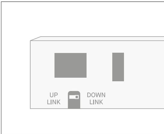
Make sure the UPLINK/DOWNLINK switch is set to the downlink position before you connect your device.
