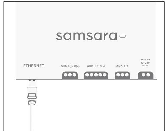
**Modbus TCP:** Connect the slave device via ethernet to the ethernet port.
