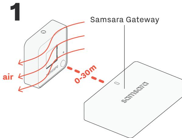
\*For optimal performance, place the device in an area with lateral airflow.
