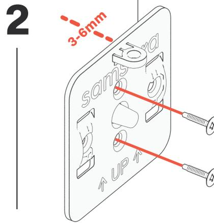
\*For optimal performance, mount the device at least 3mm away from the wall using washers.
