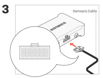
Plug the Samsara Cable gateway connector into the Gateway. It will click when fully inserted.
