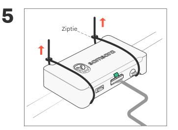
Fasten connected Gateway in a secure position behind the dashboard using zipties.
