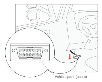
Fasten unconnected diagnostics port to vehicle's original port location.
