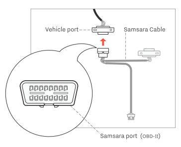
Plug the Samsara Cable gateway connector into the Gateway. It will click when fully inserted.
