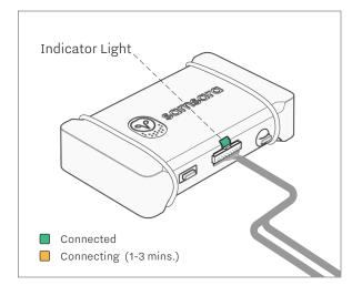
Connect the Samsara Cable. Vehicle's diagnostics remain accessible via the unconnected port.
